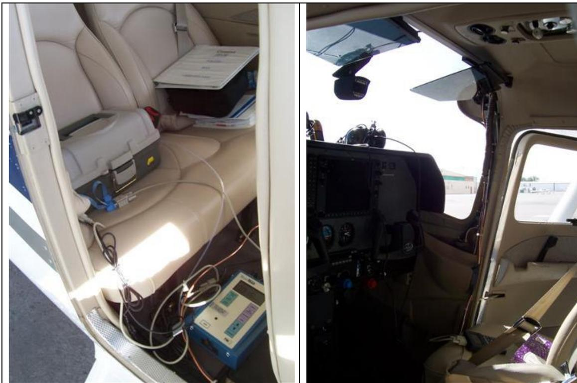
Figure 3-3. Ozone and PM<sub>2.5</sub> Sampling Package in Back Seat of Aircraft and Sample Tubing Leading Up to and Out Air Vent on the Cessna 182
