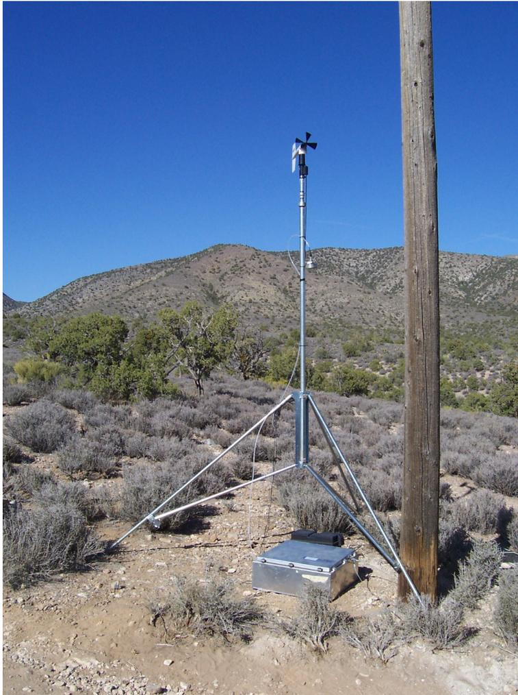
Figure 3-1. Surface Tripod Mounting of Wind Sensors, with Ozone Sampling Line – MOP Site
