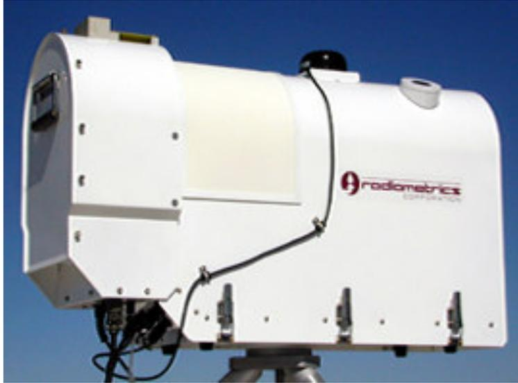
Figure 3-5. Radiometrics Profiling Radiometer
