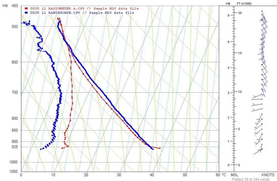
Figure 4-4. Radiometer/Rawinsonde Comparison – August 30, 1100 PST
